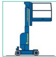
Mast 9 m height of stroke
